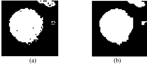
Fig. 6. Binarization. (a) binarized lumen image, (b) the hole-filling image of (a) by closing operation.
