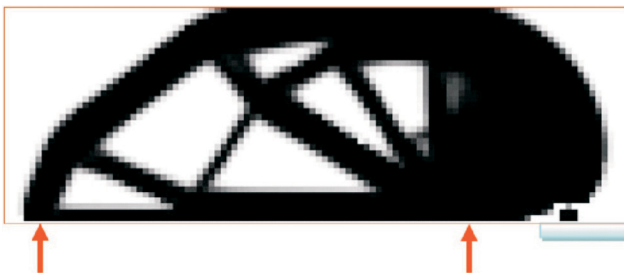
Figure 4. The final topological result of the amplifying mechanism ( V_a = 0.6 )
