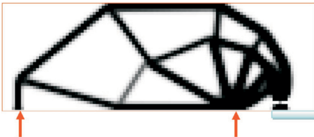
Figure 10. The final topological result of the amplifying mechanism ( V_a = 0.3 ).
