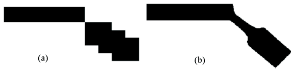
Figure 4. (a) A single-node hinge (b) Compliant hinge by post-processing [9].
