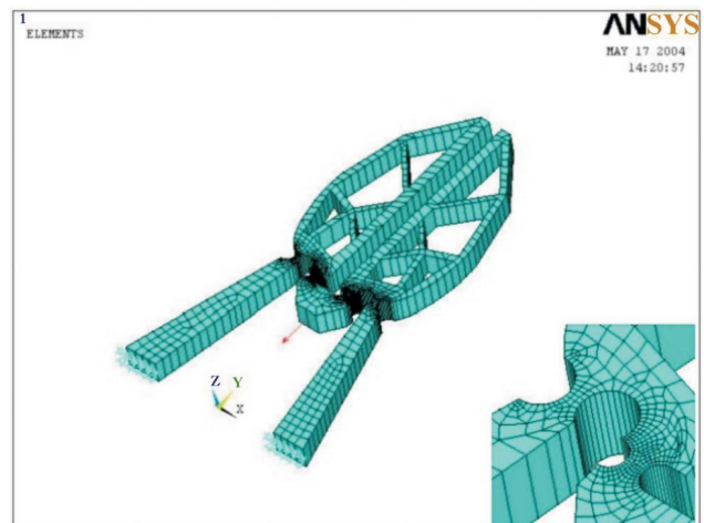
Figure 17. Finite element model for micro gripper design.
