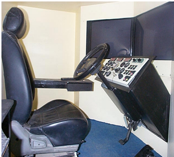
Figure 2. The dashboard inside the mockup
