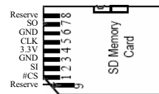
Figure 4. Schematic diagram of the memory card In this Holter recorder, a SD Card is used.
