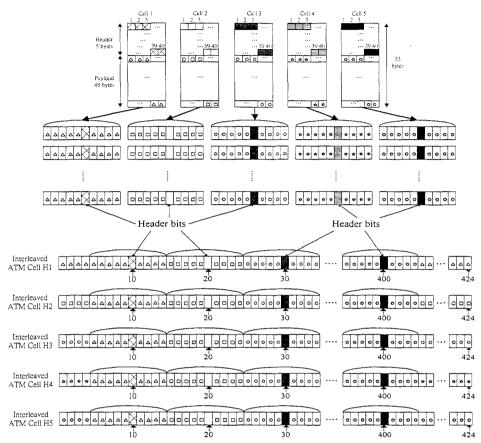
Figure 1. The bit assignment of the hyper-cells interleaving strategy (HIS).
