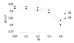
Figure 7. The received clean cell probability (RCCP) under different probability of remaining in the bad state (Ps) when P = 0.2.
