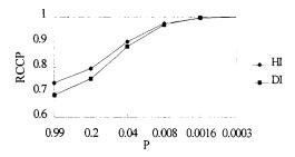
Figure 6. The received clean cell probability (RCCP) under different state transition probability from good to bad (P) when Ps = 0.9.
