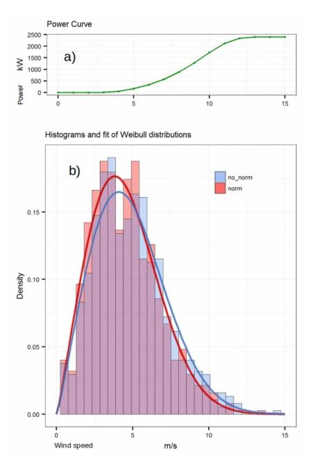
**Figure 4.** Illustration of the implementation of the wind speed distributions on the power curve of the turbine. Above (**a**), the power curve of the MWT-92/2.4 turbine is matched for the same wind speeds. Below (**b**), histograms of normalized and non-normalized wind speeds and corresponding fit of Weibull distributions during a summer with high temperatures in Cabo de Palos. Parameters: k = 2.2 in both cases; c = 5.1 (normalized distribution) and 5.5 (non-normalized).
