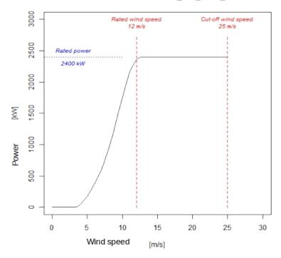
Figure 2. Power curve and characteristics of the MWT-92/2.4 turbine [40].
