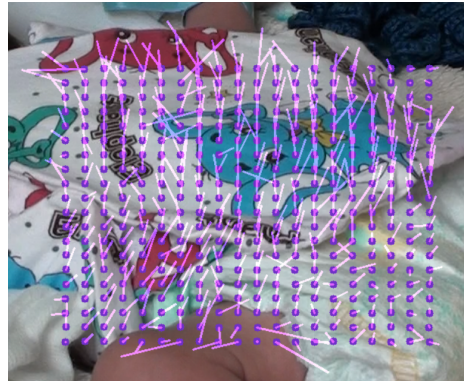
Fig. 3. An example of sparse optical flow on regular grid of image locations.
