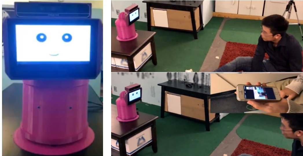
Figure 4. Companion Robot, by ASCC at Oklahoma State University (2017). Robot interface (left), and identifying a fall and video-calling for help (images on the right).
