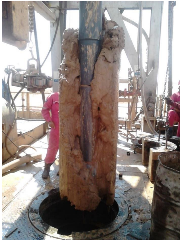
Figure 1. Hydrated clay sticks to BHA and results in a balled up bit
