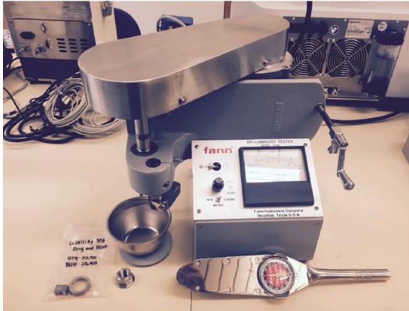
Figure 25. FANN Lubricity Tester
