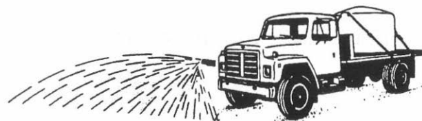
Figure 10.19 The solid-stream nozzle (a) is used for making boomless broadcast herbicide applications (b).
