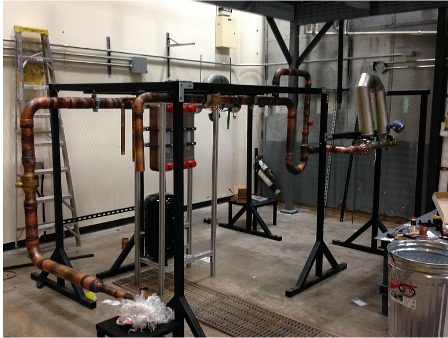
Figure 5.9: Beginning of tube assembly process as main loop tube sections are attached to the frame.
