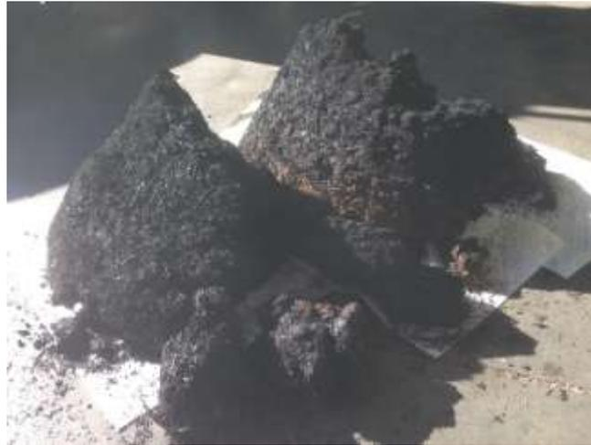
**Figure 1.13. Samples of ash/slag collected from the ash collector from co-gasification of MSW and biomass, with a detailed performance of power generation reported by Indrawan et al. [60]**
