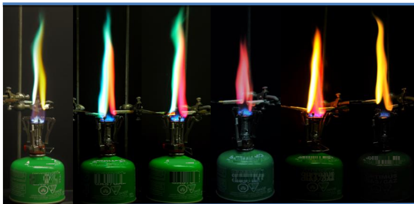
Figure 5. The mixed colored flame from saturated firebrick sticks containing \text{CuCl}_2 (blue/green)/ \text{NaCl} (yellow), \text{CuCl}_2 (blue/green)/ \text{CaCl}_2 (orange/red), \text{CuCl}_2 (blue/green)/ \text{LiCl} (fuchsia), \text{LiCl} (fuchsia)/ \text{SrCl}_2 (red), \text{NaCl} (yellow)/ \text{LiCl} (fuchsia), \text{NaCl} (yellow)/ \text{CaCl}_2 (orange/red).
