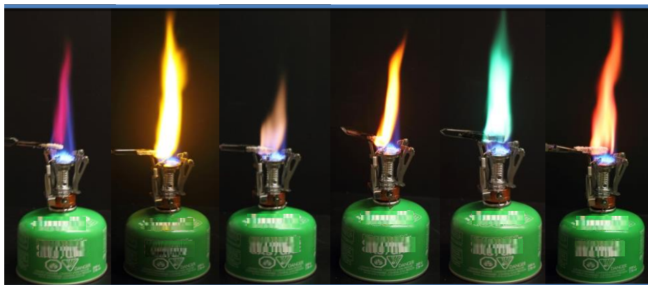
Figure 3. The colored flame in the order of fuchsia (LiCl), yellow (NaCl), lilac (KCl), orange/red (CaCl 2 ), blue/green (CuCl 2 ) and red (SrCl 2 ) (via the ultralight camping stove)
