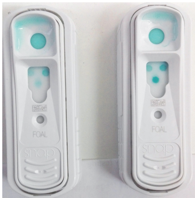
Fig. 2. Interpretation of test results less than 400 mg/dl (left) and more than 800 mg/dl (right)
