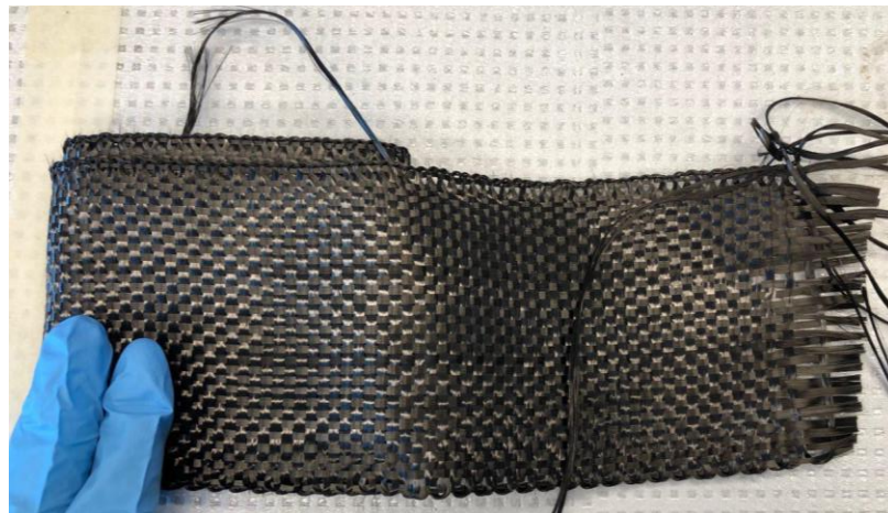
Figure 1.7: The woven carbon fiber fabrics as the reinforcement materials, fillers, before the curing process.
