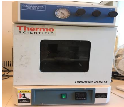
Figure 3.2: a) VBO technique using an oven and its controller b) Final cured prepreg product after using the VBO technique.
