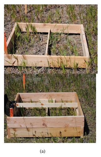
**Figure 10**. Frames designed to "mow" ROW vegetation in experimental plots so it did not exceed either (a-upper photo) 15 cm (6 in) or (b-lower photo) 30.5 cm (12 in) height.
