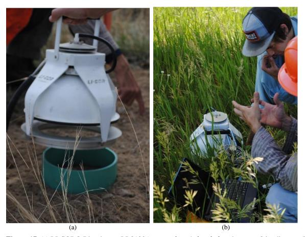
**Figure 17**. (a) LI-COR® Biosciences LI-8100A gas analyzer's hood placed over an 8 in. diameter PVC pipe that is permanently placed in an experimental plot; (b) LI-COR® Biosciences LI-8100A gas analyzer's hood placed over an experimental plot's vegetation and connected to a laptop computer as data are collected to quantify C losses from soils.
