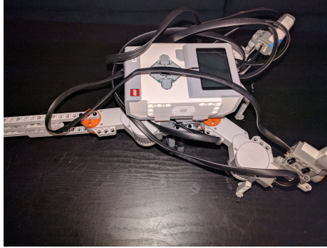
Figure 3.3: Physical robot made out of Legos. Can represent the \mathcal{M} or \mathcal{NM} robot by fixing/freeing motors.
