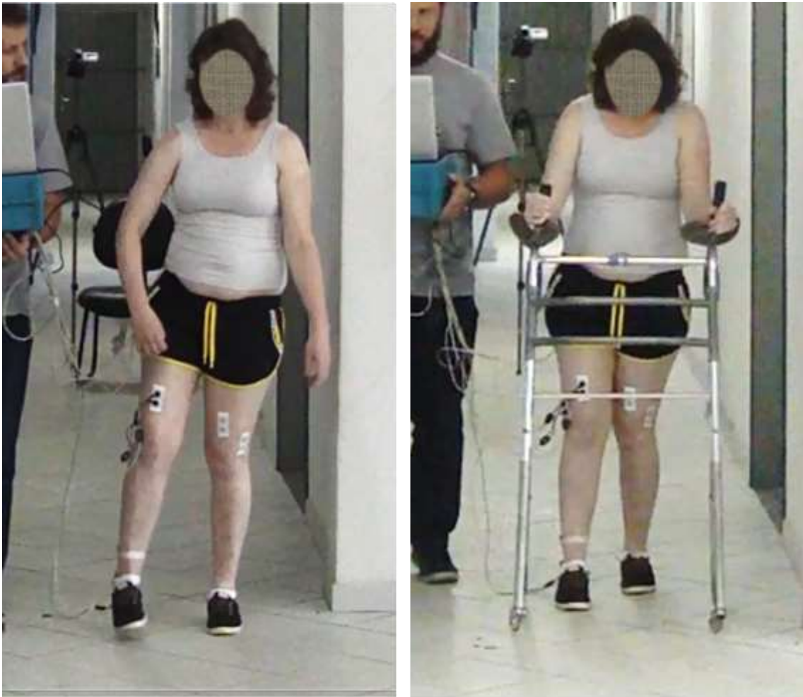
Figure 18. Volunteer, named as P2, performing the experiments of the first stage. On the left, she walks without assistance, and, on the right, she walks assisted by the modified conventional walker.
