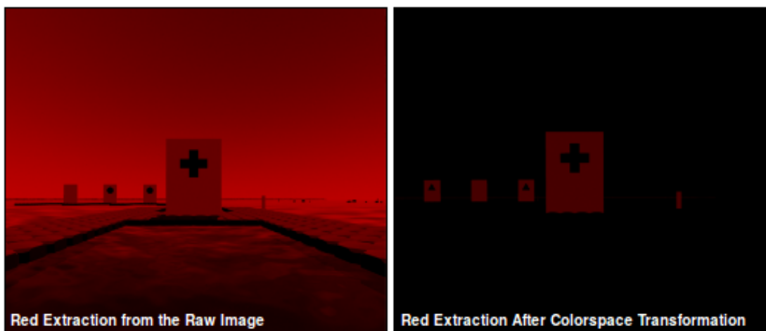
Figure 3.19: Red component extraction for both the raw image and the processed one.
