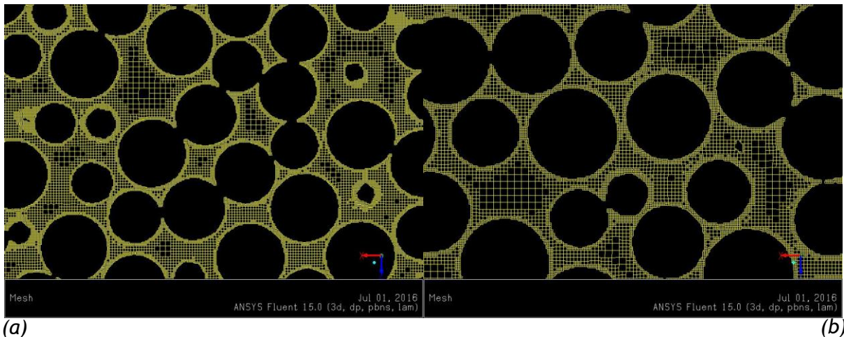
(a) Figure 10: Influence of the number of cells on the formation of bridges, left side (a) has 18 million and the right side (b) has 120 million.
