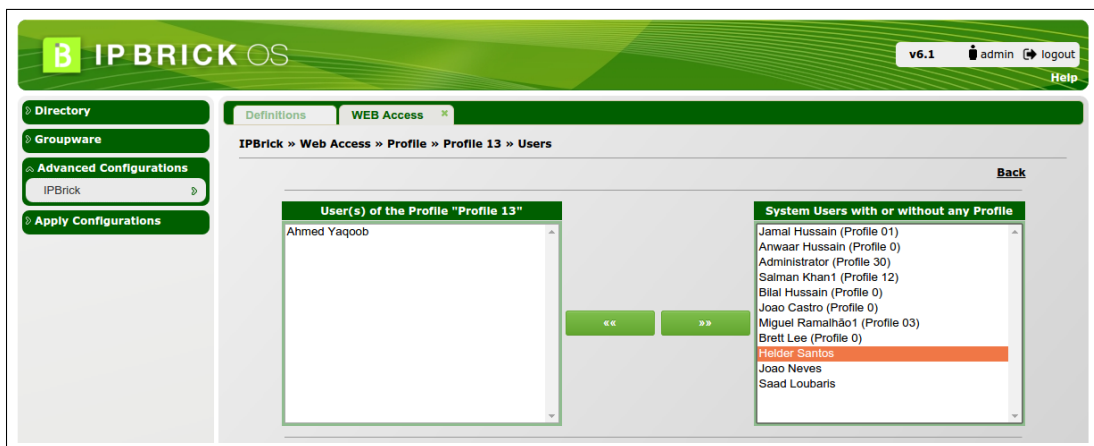
Figure 4.12: Web Page for the allocation of a user to an existing Profile
