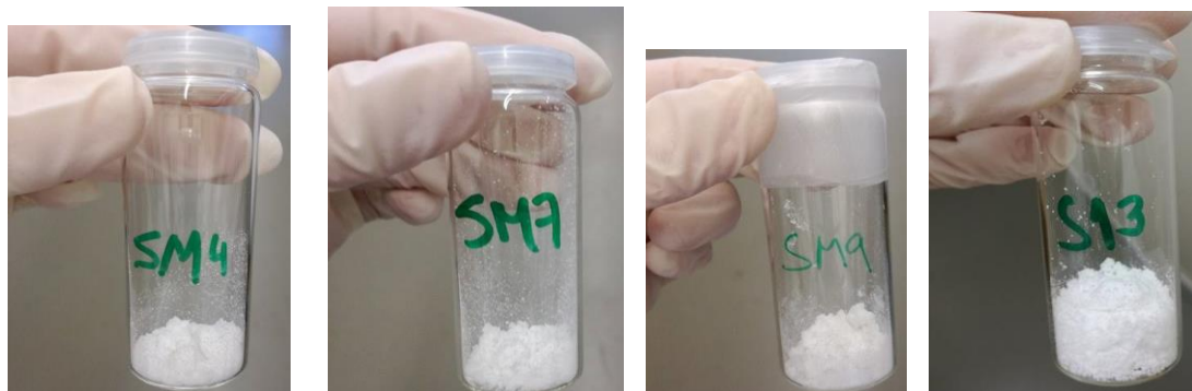
A18 - Final microparticles obtained in each individual experiment after the filtration step (examples of the four formulations, between 1 and 4, from left to right)
