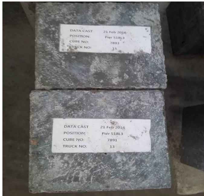
Fig.6.4 – Two concrete cubes with the correct identification
