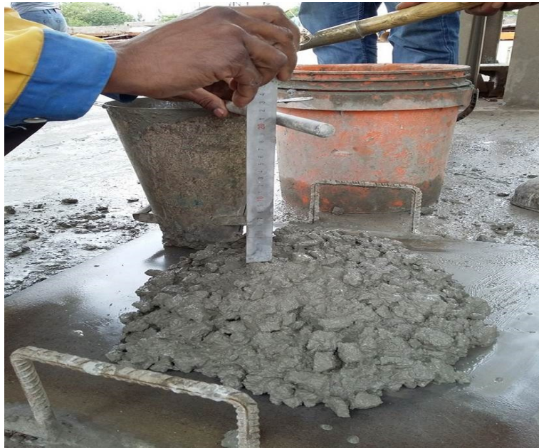
Fig.6.8 – Slump test performed for S10L1 casting
