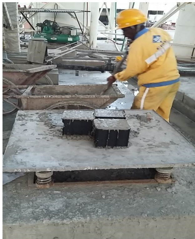
Fig.6.3 – Concrete cube samples on the vibration table
