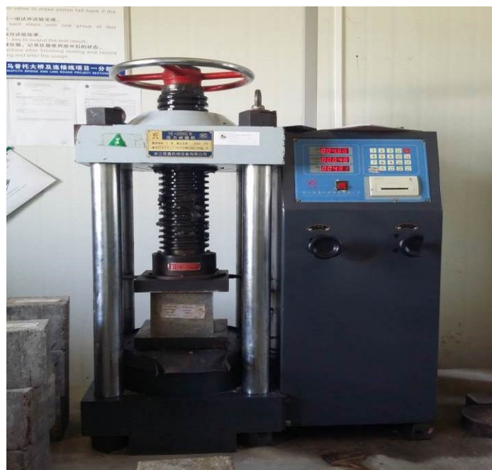
Fig.6.5 – Compressive test to determine the concrete cube strength
