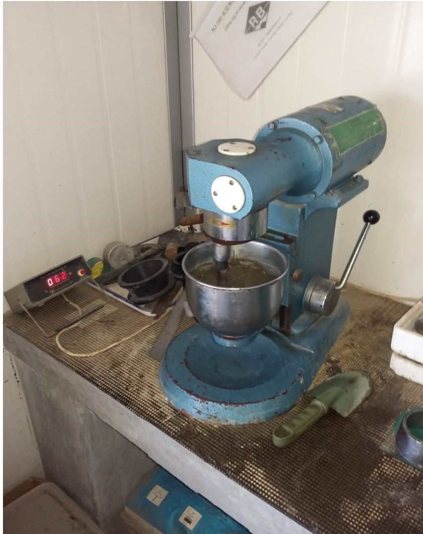
Fig.6.1 – Represents the image of a mixer used in the laboratory to mix water with cement
