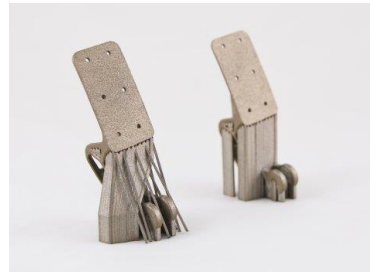
Figure 36 - Support generation using Materialise Magics SG+ module (left) and an example of produced metallic parts with the corresponding support structures (right) [42].
