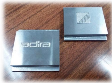
Figure 96 - Produced SLM samples on the modular test chamber. One layer was processed on top of a small metal substrate.
