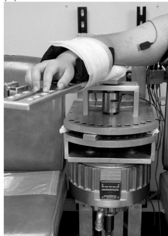
Figure 2.5: Shapiro et al. (2007) setup for rigidity quantification in the elbow joint, comprised of a motor imposing its flexion/extension. From [18].
