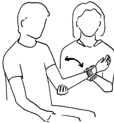
Figure 2.4: Patrick et al. setup for rigidity quantification consisting of two-force pads and a gyroscope. From [19].
