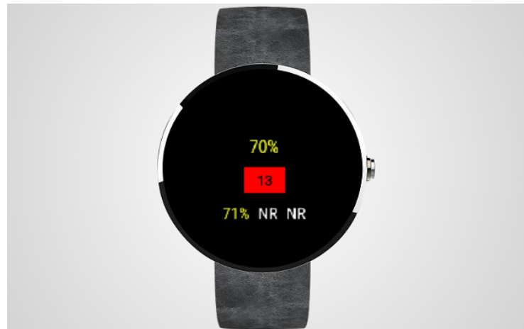
Figure 6.6: Wearable application interface in smartwatch Moto360. From top to bottom, there is the most recent rigidty label, followed by the corresponding count of cogwheel artifacts which is associated to a color code related to severity of their occurrence and, finally, the history of rigidty labels.
