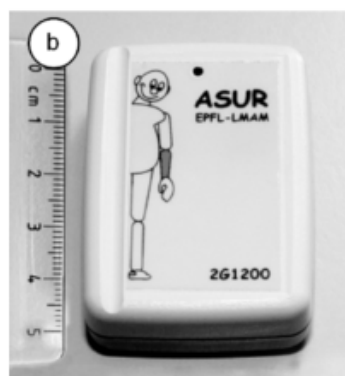
Figure 2.10: An ASUR unit developed by [28], which includes a gyroscope.
