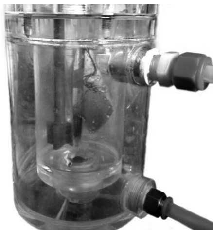
Figure 3.1 - The new electrochemical cell. a – Photo; b – Schematic cross section.
