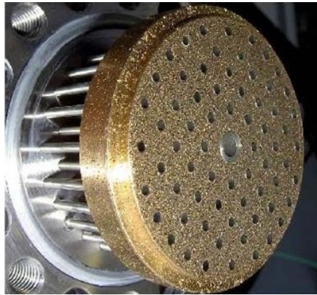
Figure 2.2: The API-68 porous injector head. [7]
