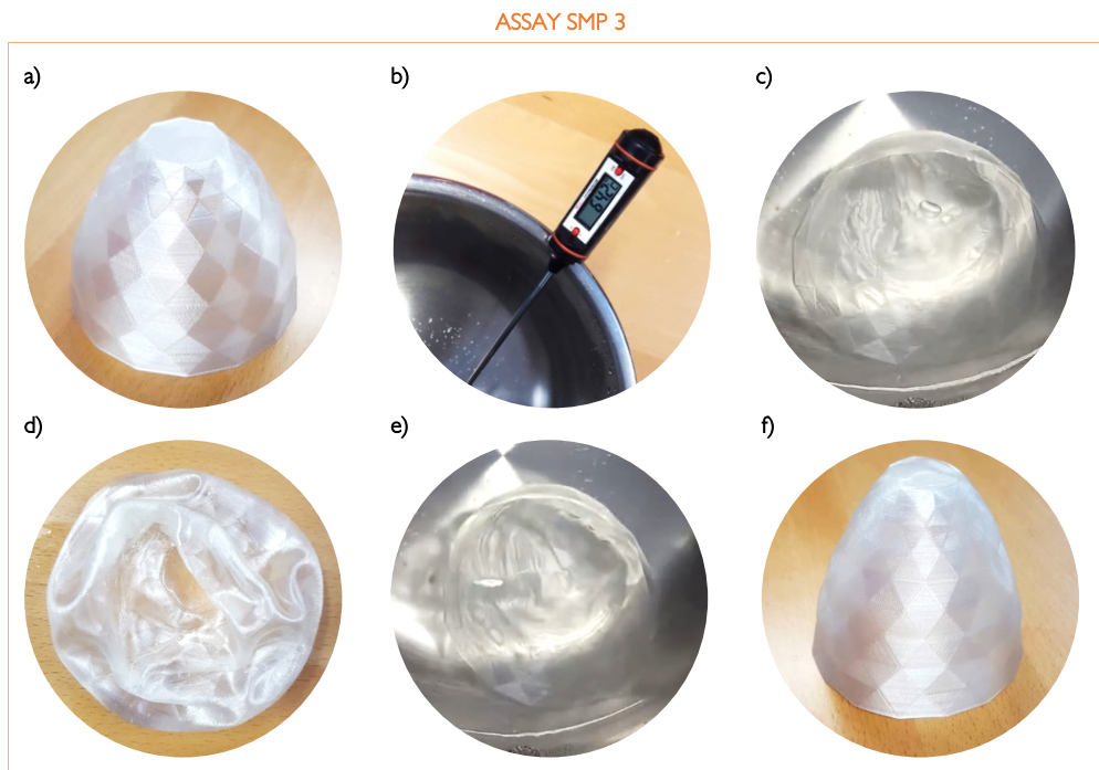
Figure 128 - Process of deformation and recovery of the sample printed from the 3D model of Figure 126. a) Printed sample with 1 mm thickness; b) Temperature control; c) Heating the sample to press; d) Pressed sample at a rigid temporary state; e) Heating the pressed sample to restore its original shape; f) Restored shape.
