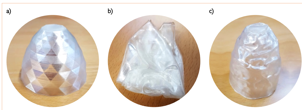
Figure 127 - Process of deformation and recovery of the sample printed from the 3D model of Figure 126. a) Printed sample using vase method (0,48 mm thickness); b) Temporary shape, folded after heated above 55°C; c) Semi restored shape.
