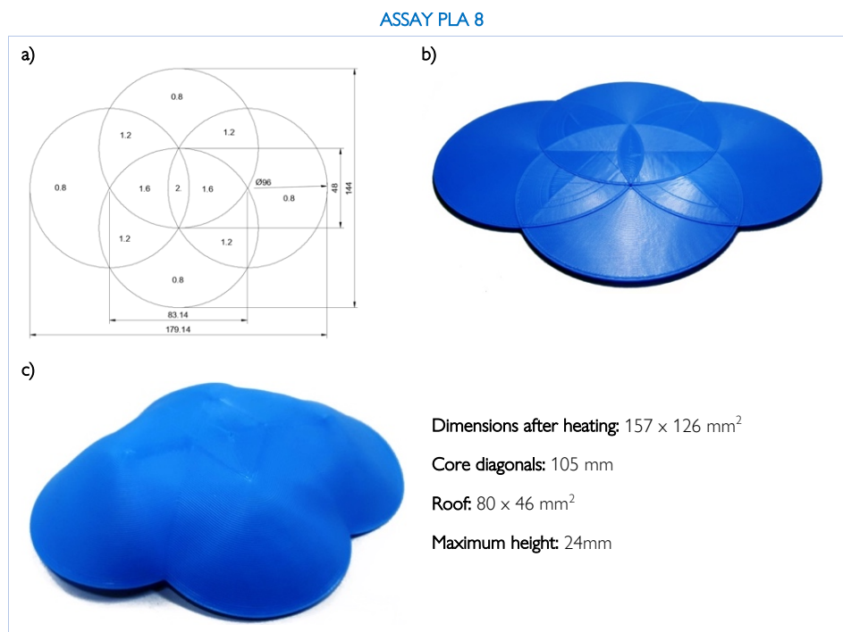
Figure 113 - Replication at scale from Figure 112. Sample with overlapping of circular sketches and thickness variation from 0,8 mm to 2 mm, the core with two crossed thickness (1,6 mm and 2 mm). a) Sample dimensions; b) Sample after printing; c) Sample after heating at 95°C and respective dimensions.
