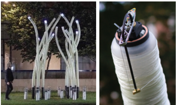
Figure 70 – An architectural-scale structure built using 16 identical Fiberbots operating in parallel over 2 days (Kayser et al. 2018)
