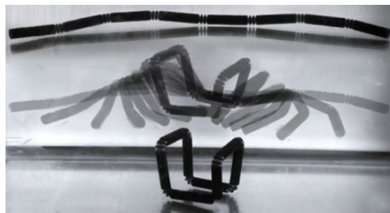
Figure 29 - 4D Concept - Transformation of 1D strand to 3D wireframe cube by self-folding after exposed to water (Tibbitts, S. 2014)
