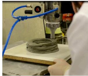
Figure 18 - 3D printing of a cylindrical tower, assisted by a turntable (Teixeira 2018)
