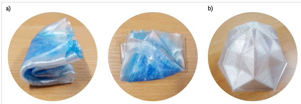
Figure 132 - Repeating the process described in Figure 131, using a PTFE sheet to assure more folds without sticking the object walls. a) Folded sample after heated, rigid temporary state; Dimensions of the folded structure: 50 x 65 x 20 mm 3 b) Restored sample to its original state.
