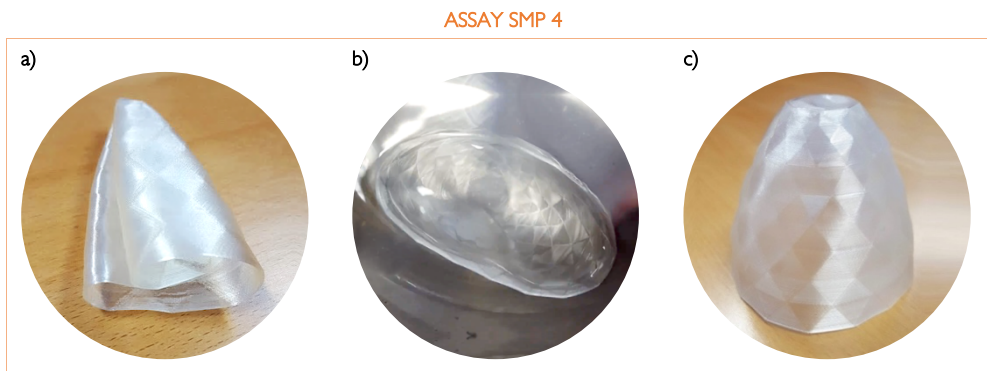
Figure 129 - Repeating the process described in assay 3 Figure 128, folding the sample instead of squeezing it. a) Folded sample after heated, rigid temporary state; b) Recovery of the sample through the immersion in hot water (above 55°C); c) Recovery sample to its original state.
