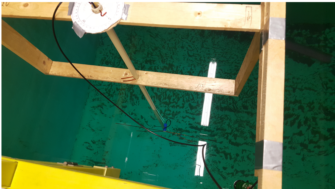
Figure 5.6: Measurement set-up for dual band dipole antenna
