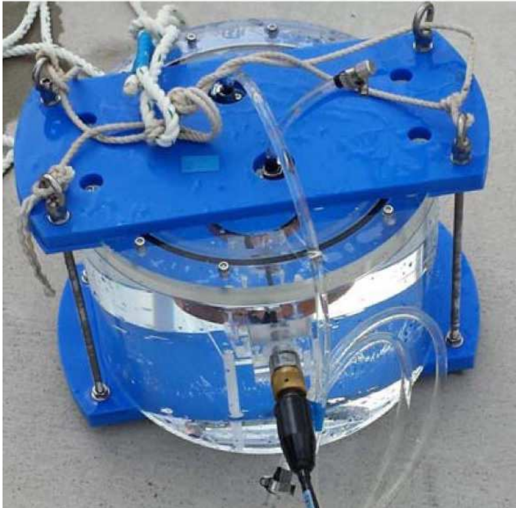
Figure 2.28: Underwater Small loop antenna in a water container [127]
