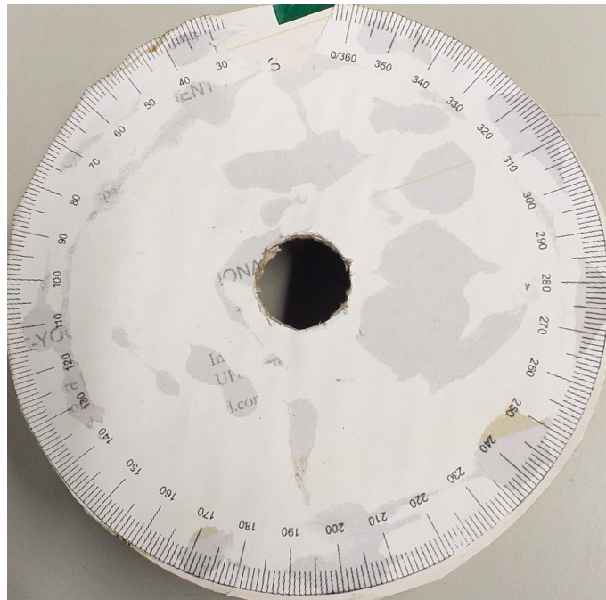
Figure 4.23: Protractor used in measurement of radiation pattern in freshwater
