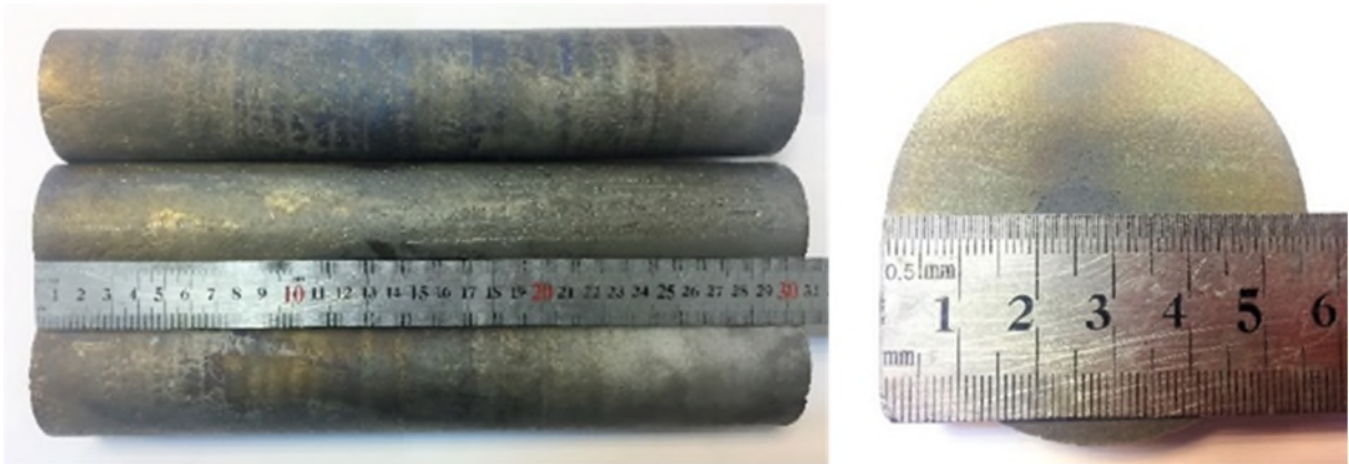
Figure 59. Cast cylindrical ingots of Ti-48Al-2Nb-0.7 Cr-0.3Si obtained via VAR.
