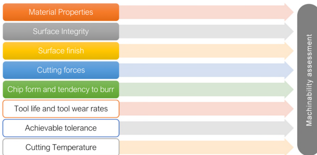
Figure 58. The most commonly used criteria for assessing machinability [64, 66].
