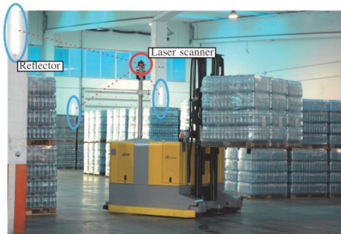
Figure 2.5: Localization using artificial landmarks. In [19].
