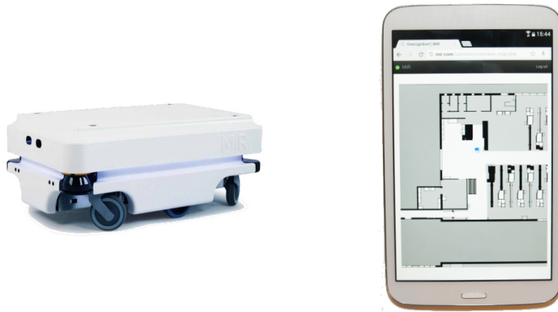
Figure 2.1: Left: The MiR100 robot. Right: Overview of a map in a tablet interface.
