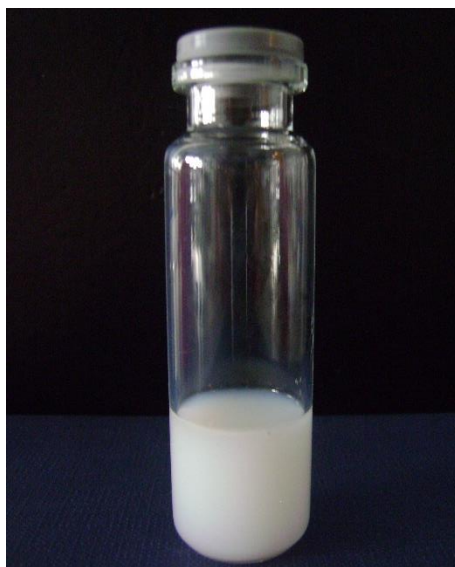
Figure 3.13: P4 formulation synthesized by double emulsion technique.
