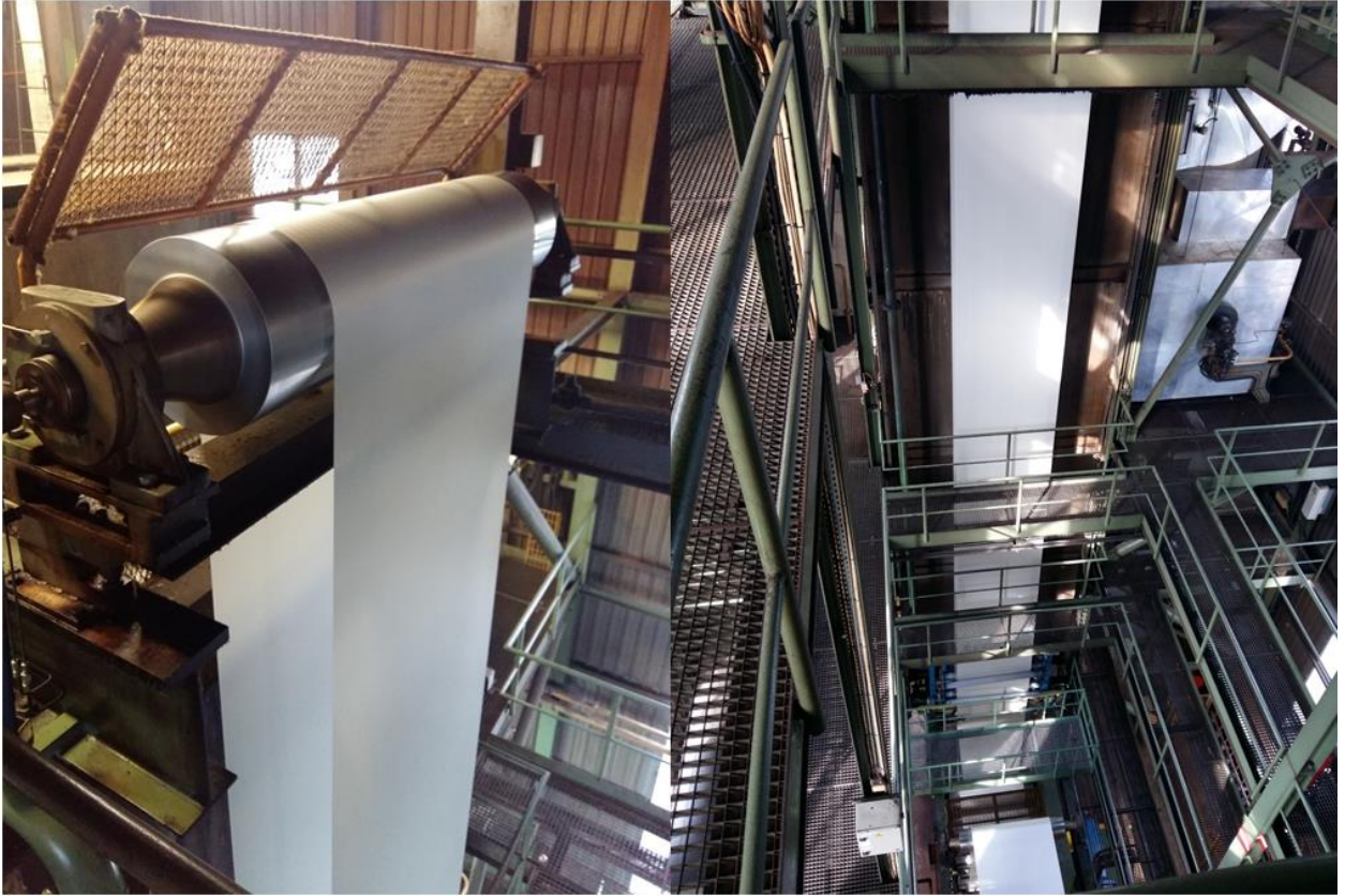
Figure 32. Path of the fabric between Oven 4 and Oven 5.
