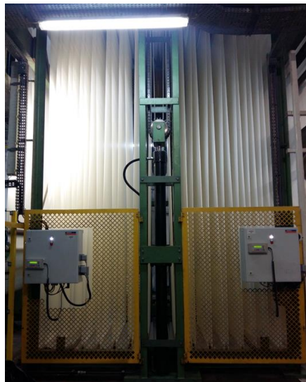
Figure 27. First fabric accumulator.
