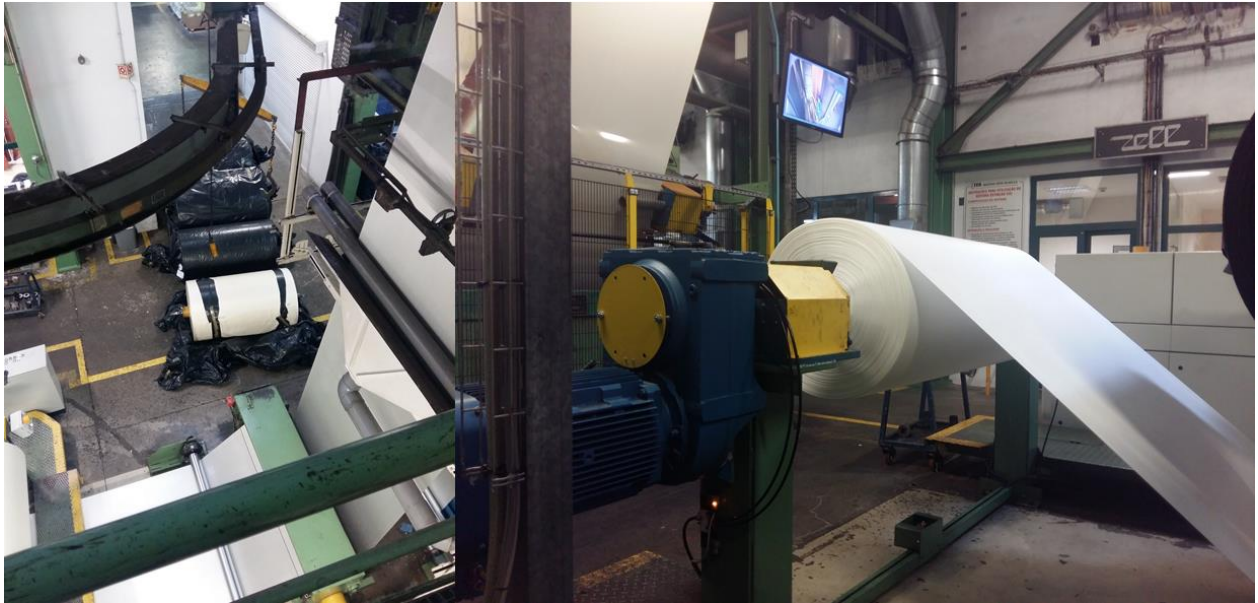
Figure 26. Supply of greige fabric and the centre driven let-off station.
