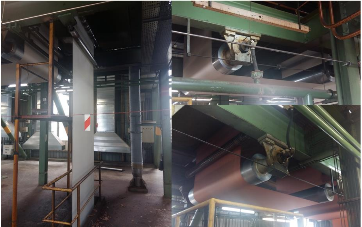
Figure 36. Fabric getting in and out of bottom of the ovens.
