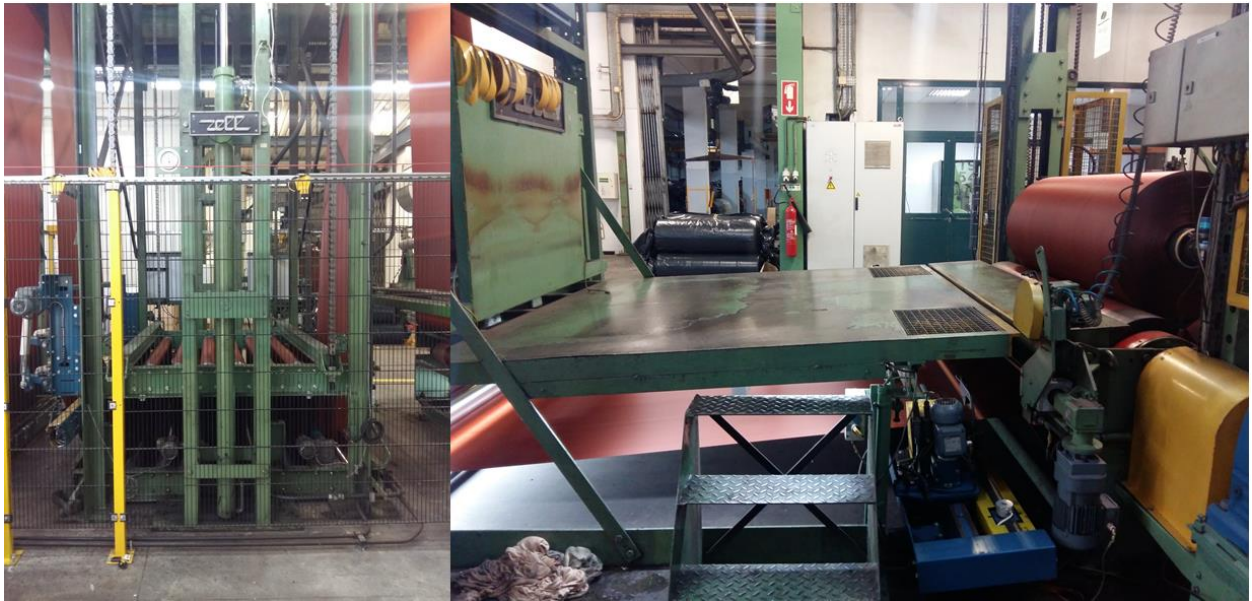
Figure 40. Second fabric accumulator and centre driven wind-up station.
