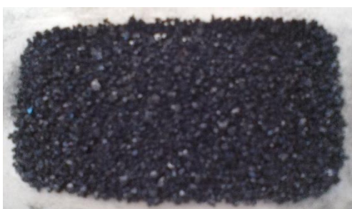
Fig. 7. Tannin-based iron-loaded adsorbent gel.
