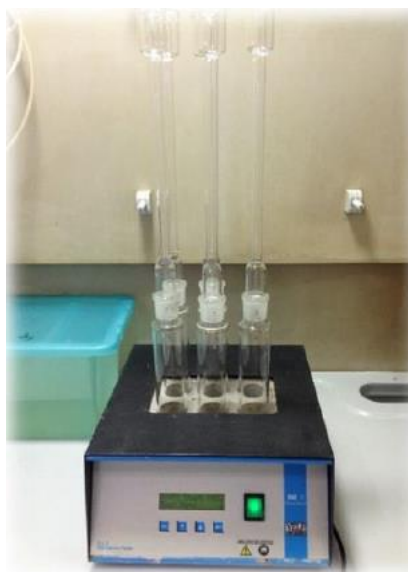
Fig. 8. Digester equipment used in the acid digestion of adsorbent samples.
