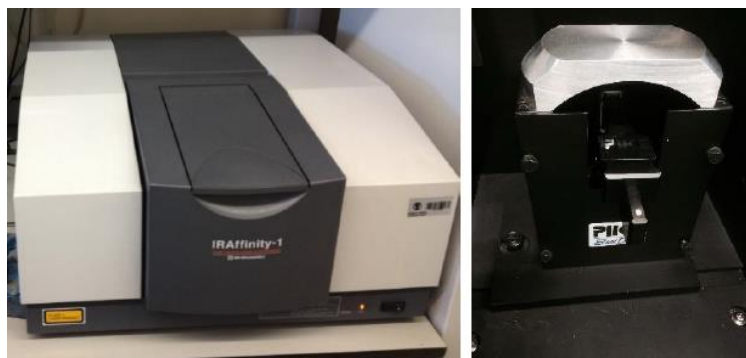
Fig. 9. FTIR spectrometer and support module for solid samples.
