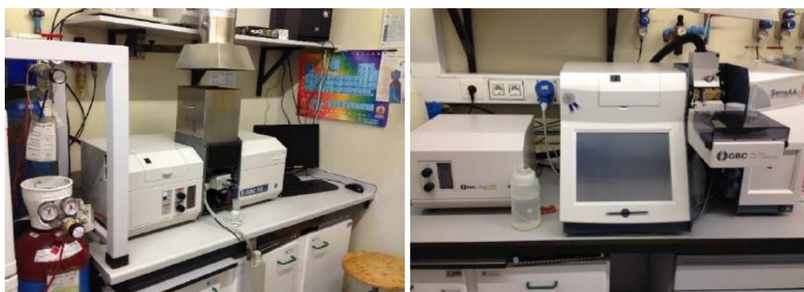
Fig. 10. Atomic Absorption Spectrometers used for As and Fe analysis: GBC 932 plus, used for FAAS determinations (left) and GBC SensAA Dual used for GFAAS measurements (on the right).
