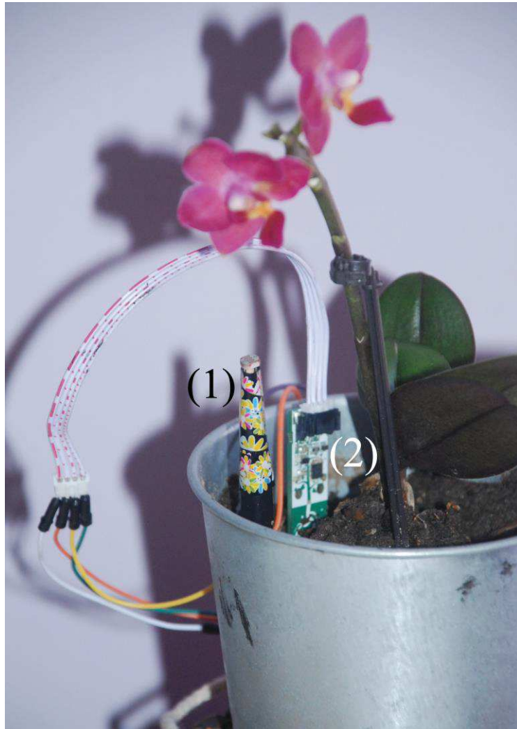
Figure 10: Detail. (1) photo-conductive cell; (2) soil moisture sensor.
