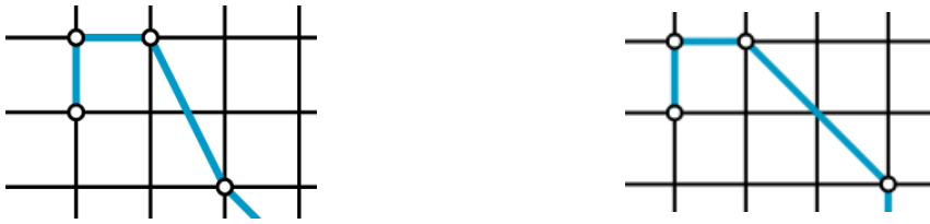
Figure 3.5: Line shape before and after the correction of a non-octilinear angle by map point displacement
