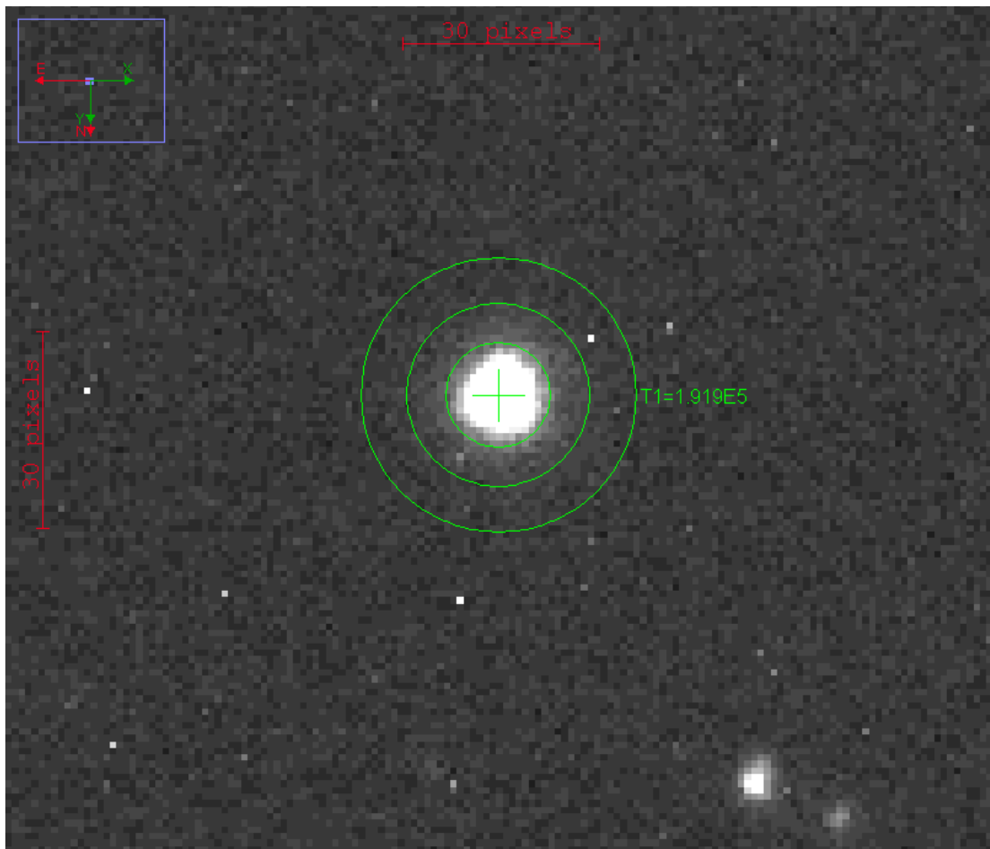
Figure 2.4. Aperture placement in AstroImageJ. The source aperture is defined by the innermost circle. Background aperture is defined as the region between the outermost and the middle circle.
