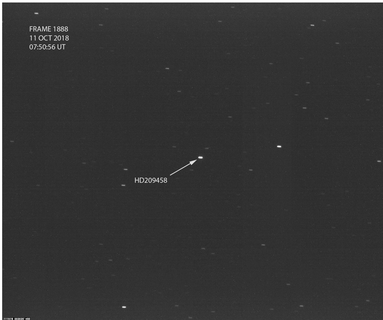
Figure 2.2. HD209485b discarded frame showing excessive mount movement. Stars appear as horizontal smears across the sky instead of well defined points of light.
