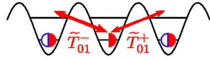
FIG. 2. Visualization of the direction-dependent interband density-dependent tunnelings in the dressed picture. The dressed tunneling amplitudes are direction dependent.
