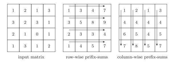
Figure 3.1: Row-wise and column-wise prefix-sums of a  $4 \times 4$  matrix
