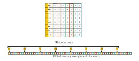
Figure 3.5: Stride access to the global memory (CUB-prefix for each column)
