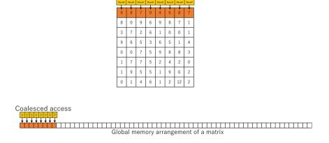
Figure 3.2: Coalesced access to the global memory (the column-wise prefix-sums)
