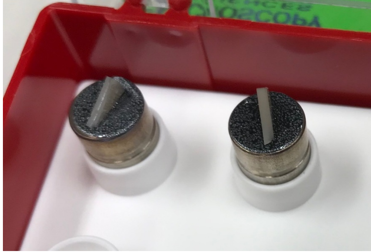
FIGURE 17. Gold sputter coated specimens ready for SEM imaging.
