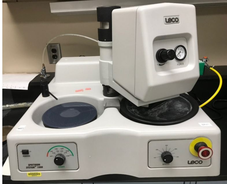
FIGURE 5. Leco polisher used to polish specimens up to 1200- \mu\text{m} grit.
