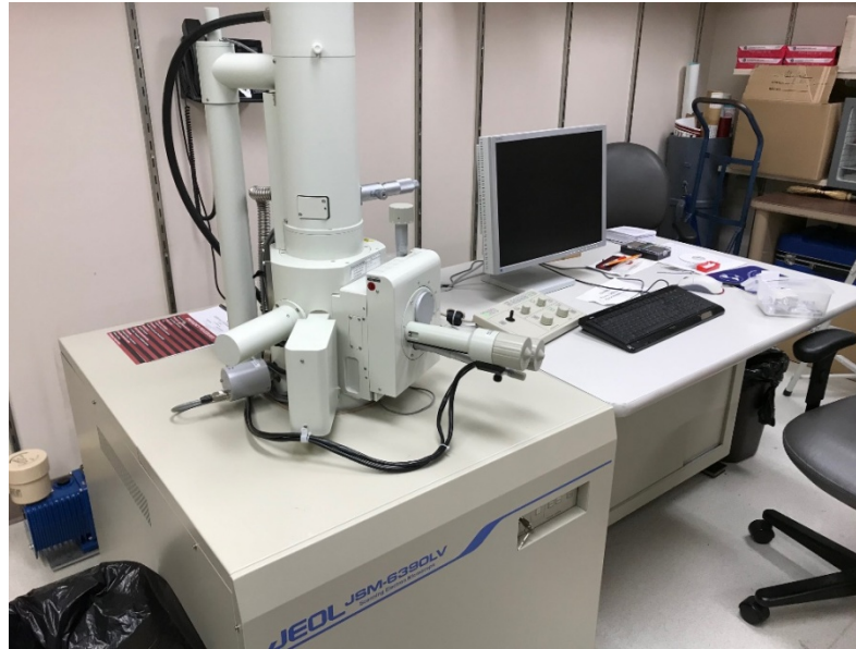
FIGURE 15. JEOL JSM-6390LV scanning electron microscope.
