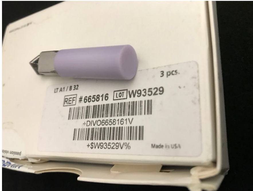
FIGURE 3. Lathe-cut (to create cylinder shape) 32-mm long e.max CAD block 12-mm wide for specimens ready to cut.
