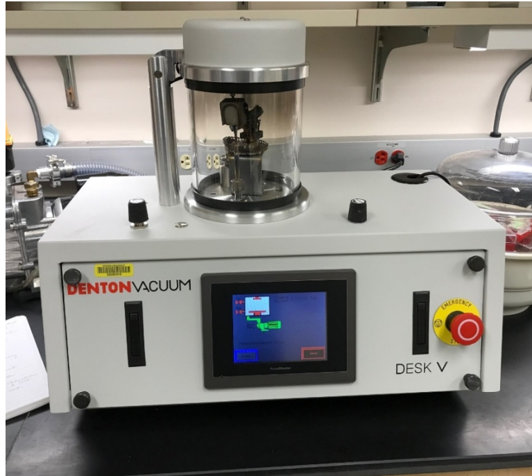
FIGURE 16. Desk V, Denton Vacuum sputter coat machine.
