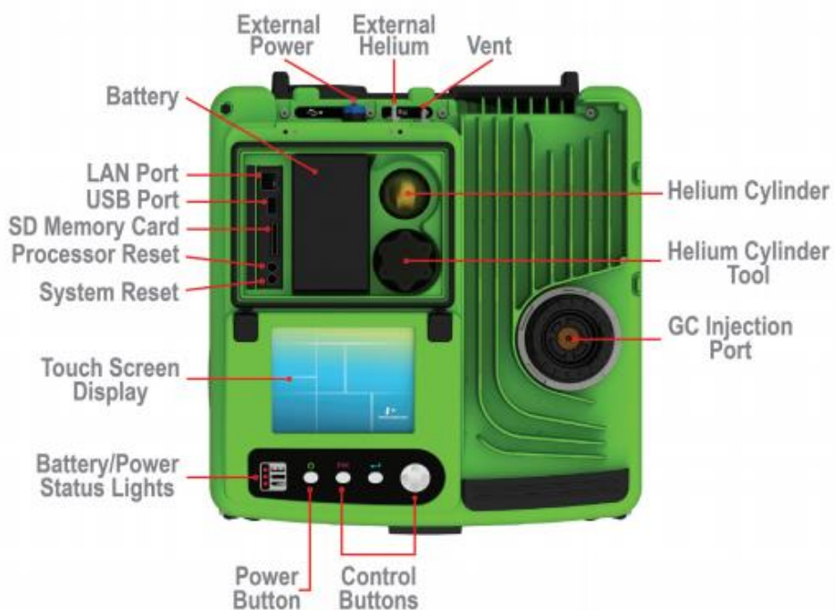
Figure 4-3. Top view diagram of a Torion T-9 portable GC-MS 55
