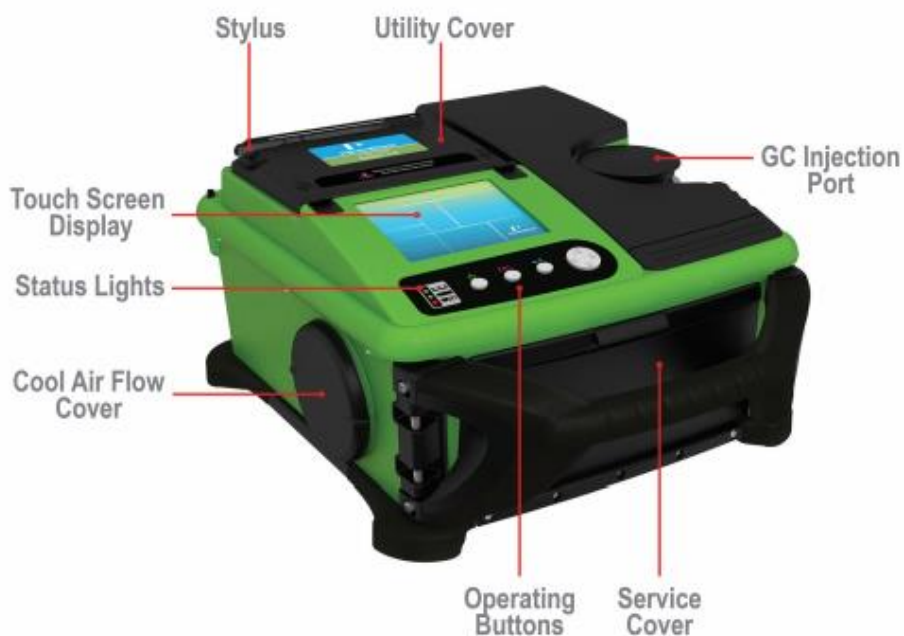
Figure 4-2. Diagram of a Torion T-9 portable GC-MS 55
