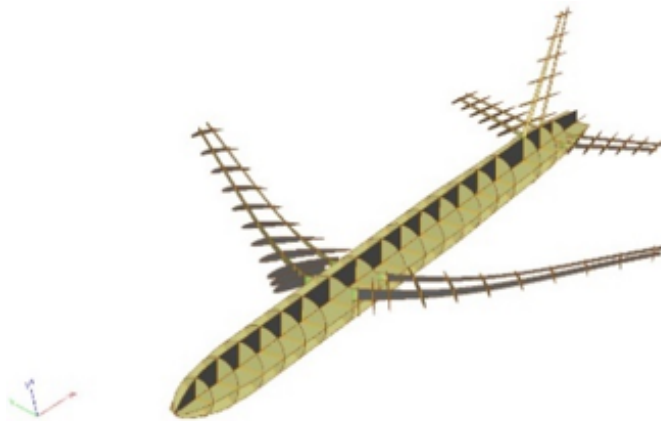
Fig. 2.4. The internal structure with the stringers unioned.
