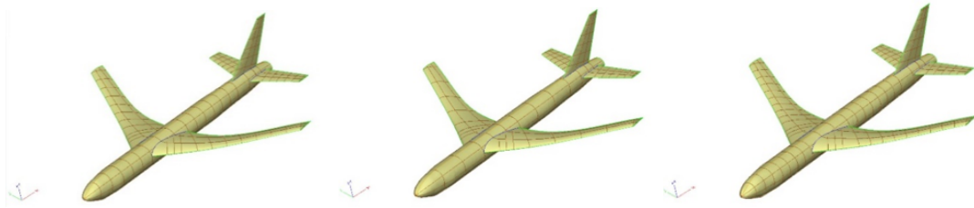
Fig. 2.7. Parametric generation of the OML and the internal structure of a commercial plane in ESP.
