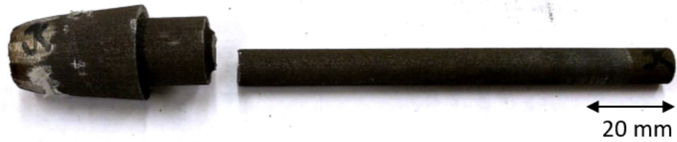
Fig. 3.6. The specimen after fatigue failure
