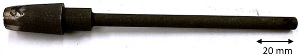
Fig. 3.2. 15-5 PH rotating bending specimen
