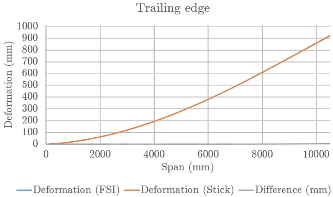
Fig. 3.18. Deformation vs Span at Trailing Edge (Alfa = 7)
