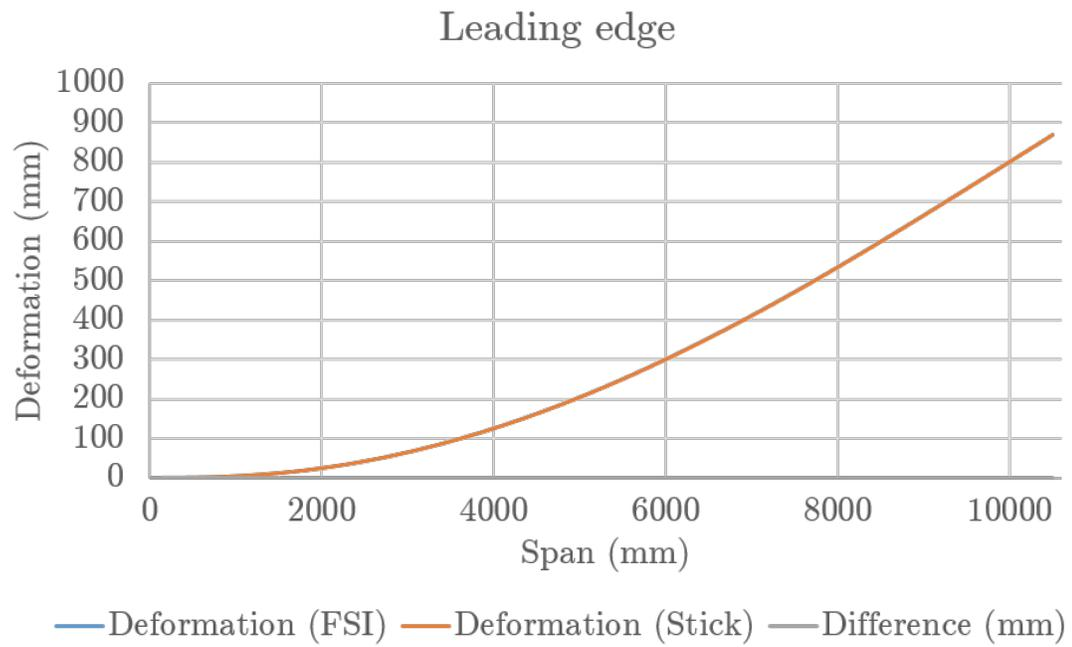
Fig. 3.17. Deformation vs Span at Leading Edge (Alfa = 7)
