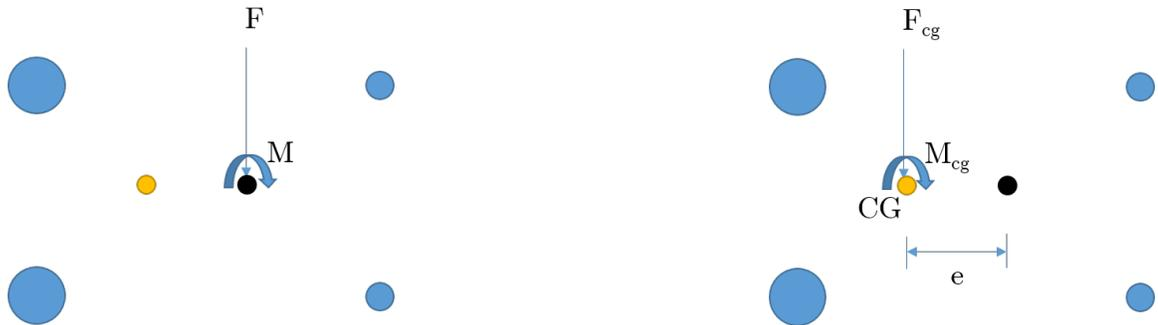
Fig. 2.4. Load Transfer to CG
