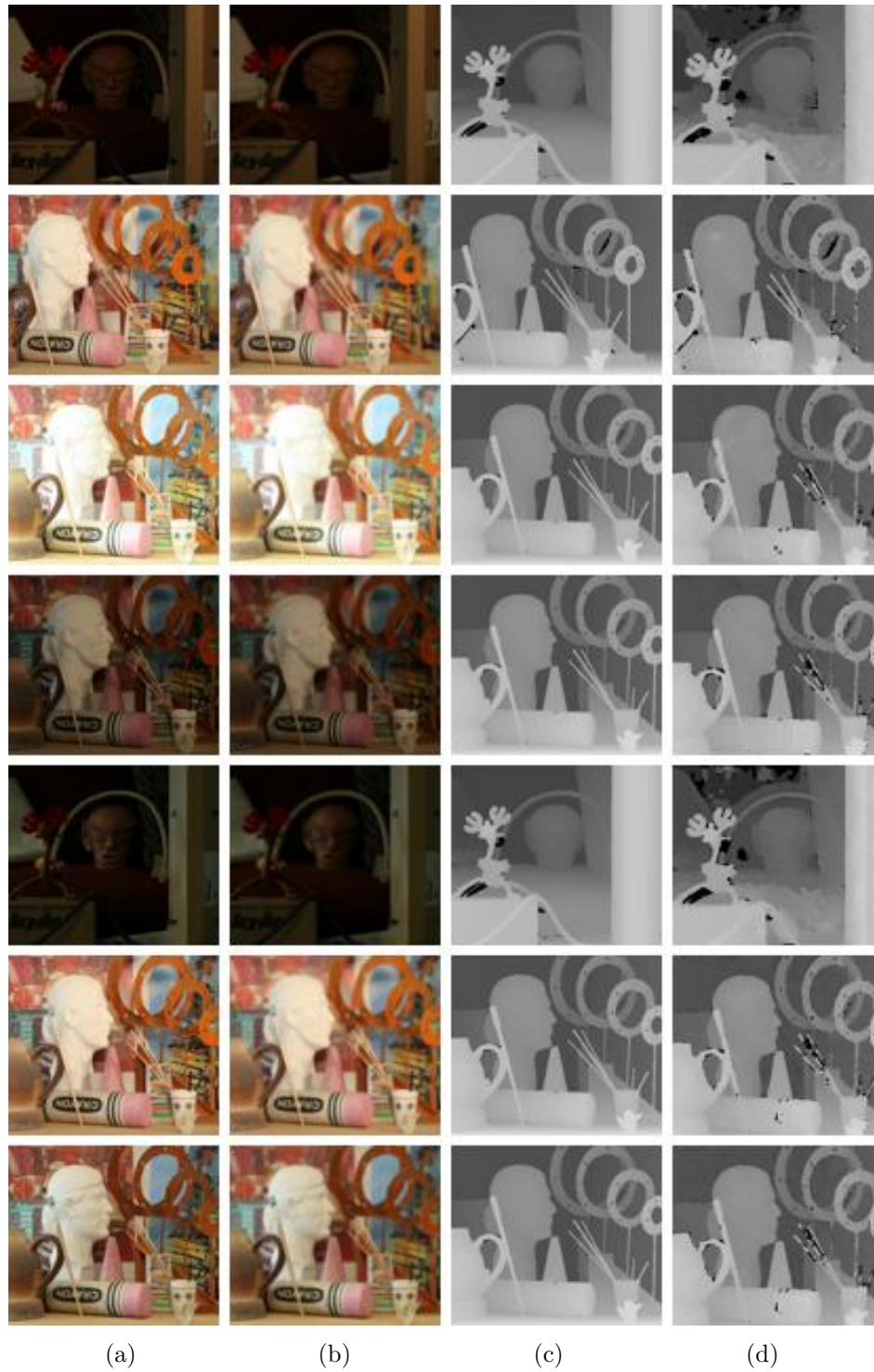
Fig. D.7. Filter Reduction Performance Results for the Middlebury College Dataset - Part 6. (a) In-focus Image, (b) Out-of-focus Image, (c) Ground Truth Depth Map and (d) DfD-Net Computed Depth Map.
