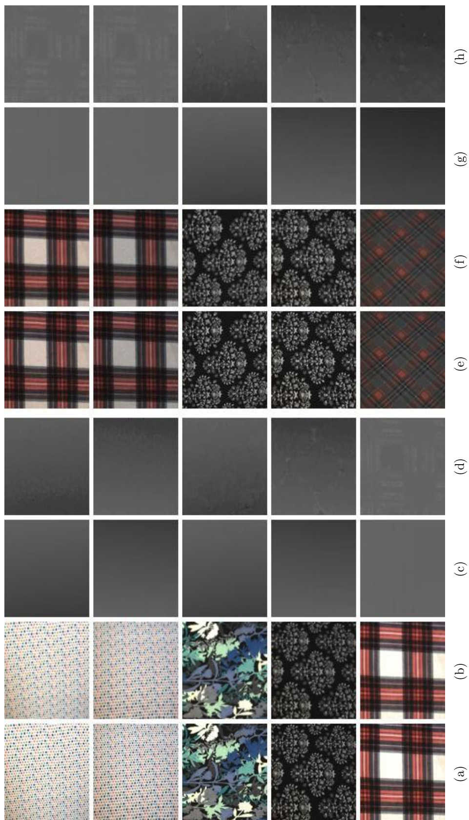
Fig. E.21. K01-K03 Scene Type Performance Results for the DfD-Net on the Synthetically Blurred Real World Dataset - Part 20. (a) & (e) In-focus Image, (b) & (f) Out-of-focus Image, (c) & (g) Inverted Ground Truth Depth Map and (d) & (h) DfD-Net Computed Depth Map.
