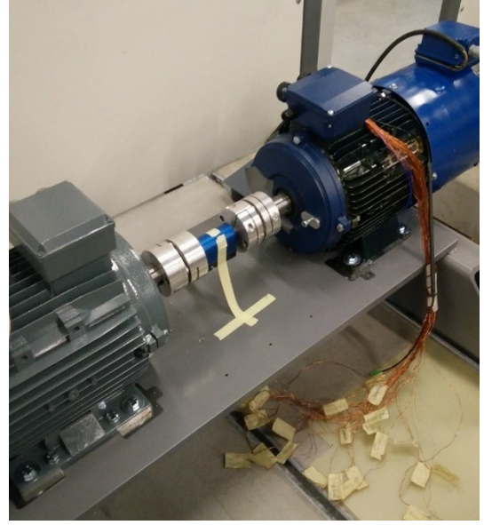
Fig. 1. Illustration of the experimental setup: the blue 5.5 kW test motor on the right is connected directly to a 3-phase 400 V main grid and runs in a no-load condition, while the motor on the left is not powered. The coated copper wires coming out of the right motor are the lead wires of the temperature sensors embedded in the windings of the machine (see Fig. 2 for sensor locations).
