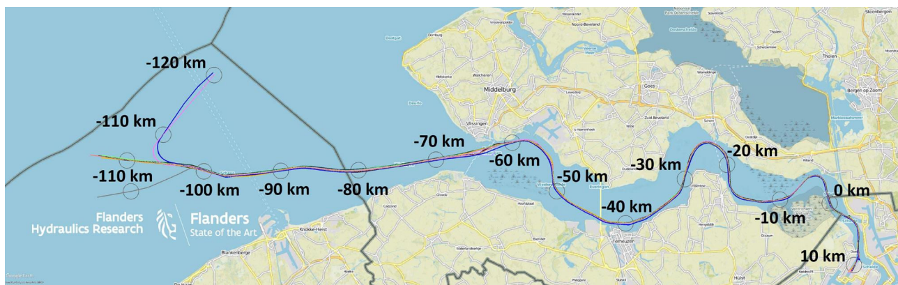
Figure 2. Trajectories for nine container vessels with running distances (colour code see Table 1)
