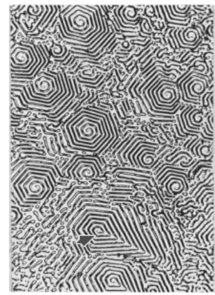
(f) Typical microstructure of Zn-3%-Mg alloy. [13]
