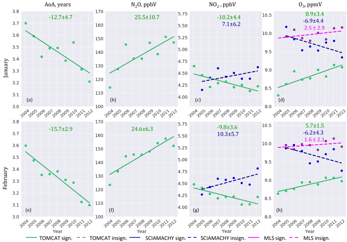
Figure 10.12: Linear changes in AoA, N 2 O, NO 2 , and O 3 with extracted QBO effect averaged over (a-d) Januaries 2004-2012 and (e-h) Februaries 2004-2011 in the tropical middle stratosphere. Colour coding indicates the data source: TOMCAT CNTL simulation (green), SCIAMACHY (dark blue), and MLS (magenta) measurements. Solid lines indicate statistically significant linear changes, dashed lines indicate statistically insignificant changes. Colour-coded trend values and their errors (in % per decade) are shown in each panel.
