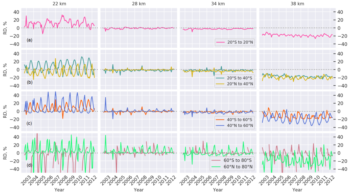
Figure 9.3: Time series of the RD of retrieved \text{NO}_2 from SCIAMACHY IUP V4.0 and V3.1 for four different altitudes, from left to right: 22, 28, 34, and 38 km. Colour coding indicates the RD at particular latitude band: tropics - magenta, middle latitudes I SH - dark green, NH - yellow, middle latitudes II SH - orange, NH - blue, high latitudes SH - dark pink, NH - light green.
